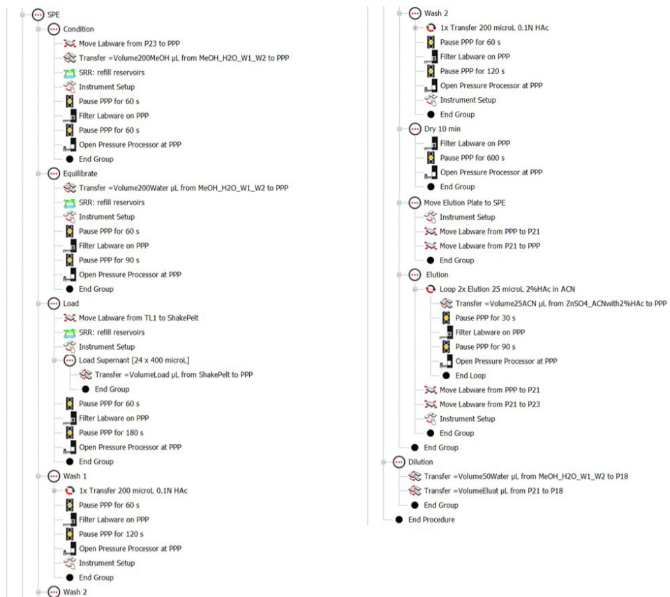
Figure 5. Biomek i7 method for THC determination – Sample cleanup using SPE.
